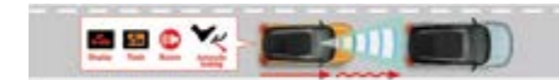
Applies strong automatic braking if the risk of collision increases even more
