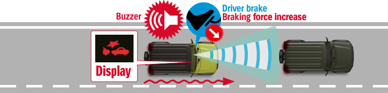
2. Deploys brake assist to increase braking force if the risk of collision is high and the driver panic brakes.
