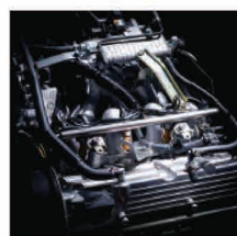
1.6 Liter, 4 Cylinder SOHC 16V Engine
