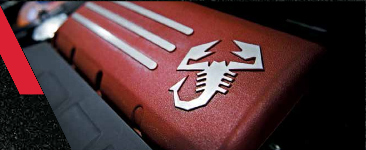
T-Jet engine 4-cylinders, 1368 cm 3 .
