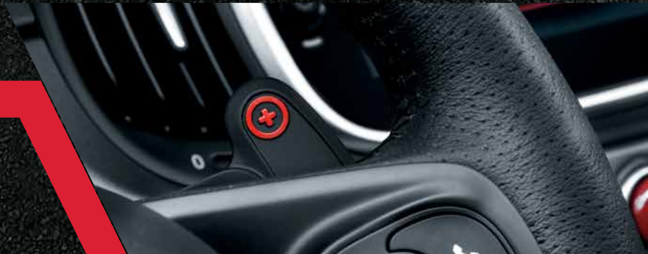
Sequential robotised gearbox with shift paddles.
