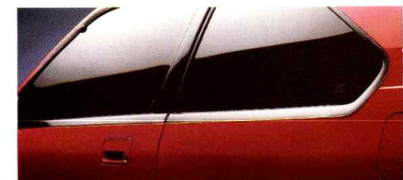
Flush-fit windows enhance aerodynamics.
