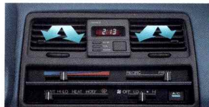
Air Conditioner. Circulates air evenly and efficiently. Also works with the heater providing de-humidified air on damp winter days.
