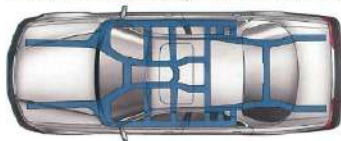
THE FULLY BRACED STRUCTURE OF THE LEGEND UNITS OFFERS EXCELLENT FRONT, REAR AND SIDE OCCUPANT PROTECTION.
