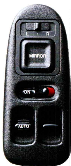
In all Integra models, the ergonomically designed control panel located in the driver's side front door handle, houses power controls for windows and door mirrors.
