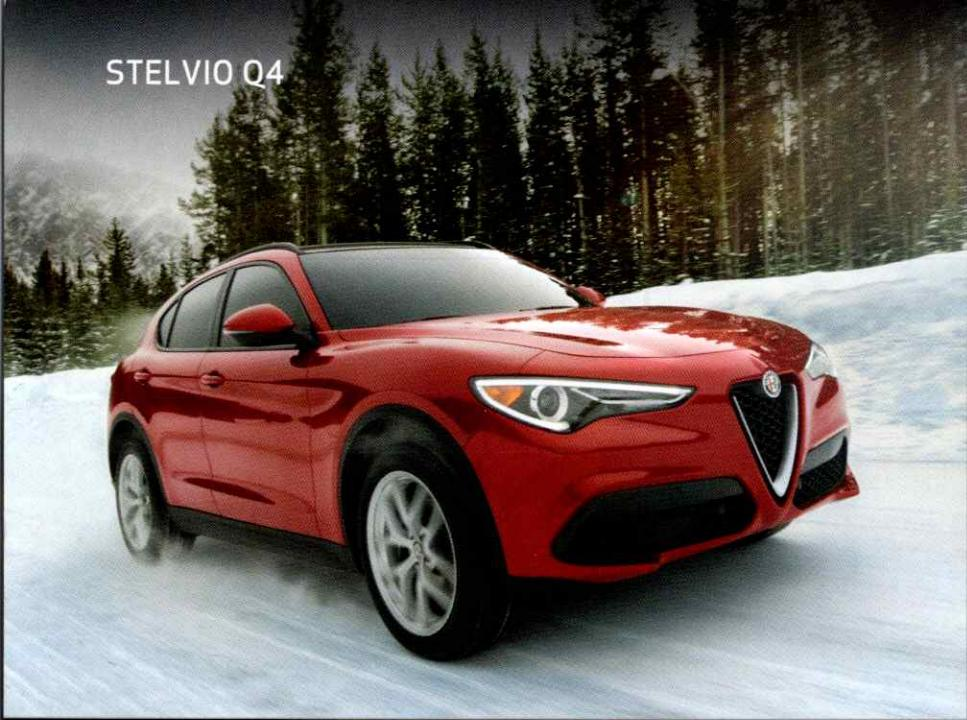
**STELVIO** features the Q4 All-Wheel-Drive (AWD) system, which transfers up to 60% of the torque to the front axle for ultimate responsiveness and stability. This all-weather confidence begins with the Chassis Domain Control (CDC), which integrates all the active systems while the Active Transfer Case (ATC) continuously monitors road conditions. Performance is further enhanced with an Integrated Brake System (IBS), Electronic Stability Control (ESC)<sup>6</sup> and Stop/Start technology.
