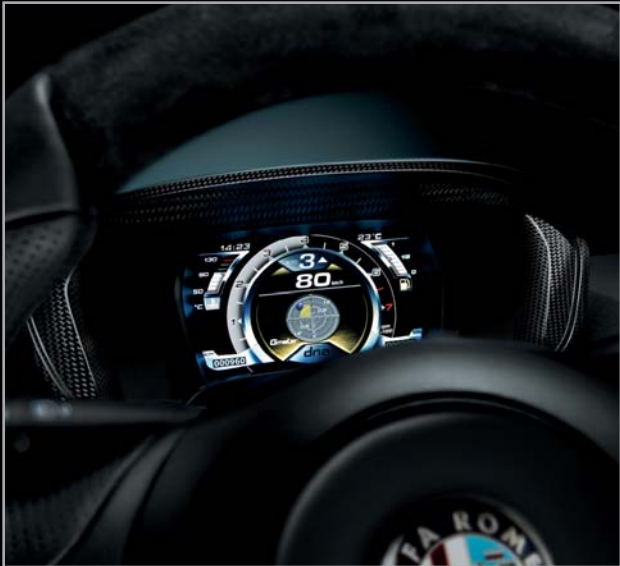
Full digital instrument panel with TFT technology Carbon fibre instrument panel fairing
