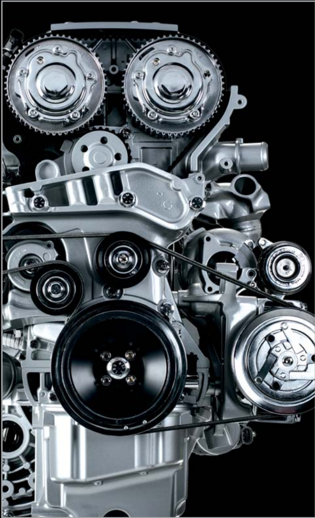
1750 cc, aluminium, 4 cylinder, turbocharged engine
