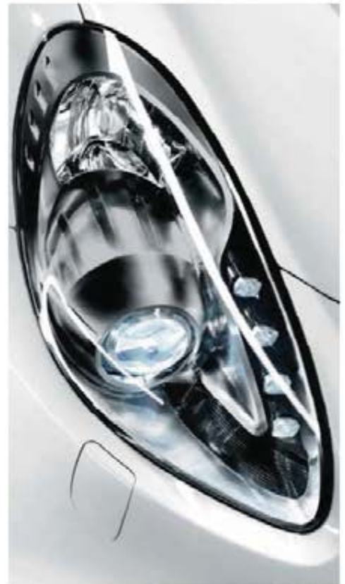
Bi-Xenon headlights with AFS and headlight washer system (opt)
