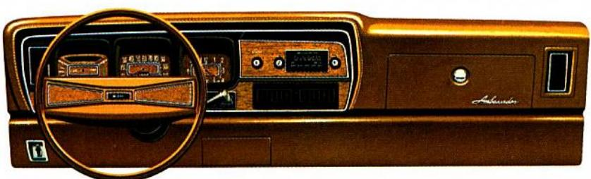
The deep-padded woodgrained instrument panel has been designed for maximum driver safety and convenience. Controls and instruments are easily accessible and easy to read.
