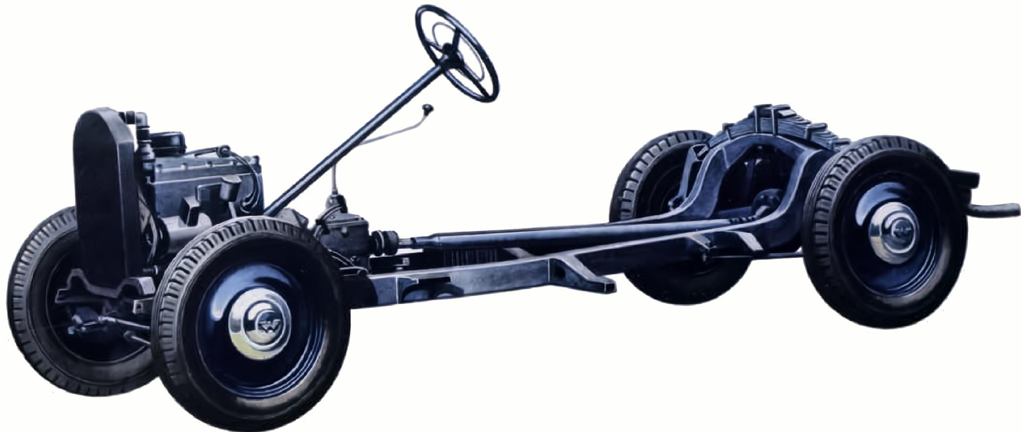
free load which thus ensures a hitherto unknown degree of stability in cornering, besides great safety in driving. The method of "floating axle" (a copyright owned by the Auto Union), has already been applied in practice to many other types of cars of the Auto Union (for inst. WANDERER Compressor).
