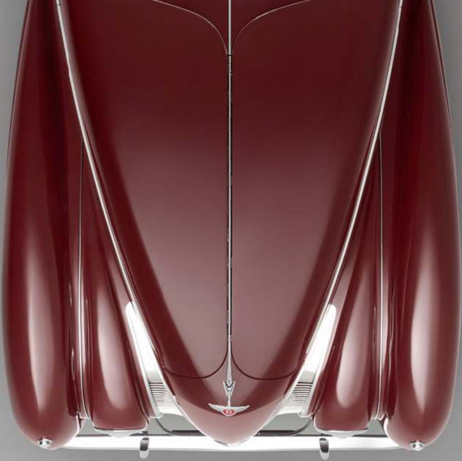
Equipped only with the original prototype's technical drawings and a handful of its surviving mechanical components, the Mulliner Classic team had to completely remake the sleek bodywork from scratch. The goal was to cleave faithfully to the lost 1939 car in every aspect, from the specially mixed Maroon and Heather Grey paint finish and unique interior trim to the tool tray and tread plates. The incredible one-off result is now a permanent resident in Bentley's Heritage Collection.
