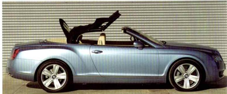
The roof comes with a heated glass rear window and also an interior roflamp in the headlining. It can be operated after pulling away from standstill at speeds up to 30km/h (20mph).
