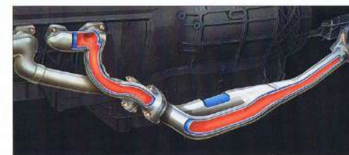
The new double-wall exhaust system featured on the 8-cylinders ensures optimum catalytic converter efficiency almost immediately after the engine starts running.
