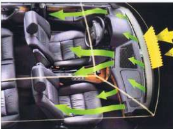
Air drawn from the outside passes through a micro-filter that removes pollen, dust particles and even some bacteria.
