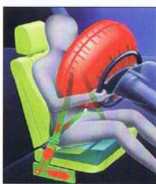
BMW's dual airbag supplemental restraint system — standard for both driver and front passenger — inflates within split-seconds, and a sensor unlocks all doors and switches on the interior lights.
