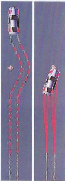
Standard on all BMWs, a four-sensor anti-lock braking system (ABS) offers added safety in emergency braking. ABS prevents wheel lock-up under hard braking, allowing the driver greater control in avoiding objects and the ability to drive out of potential accidents.
