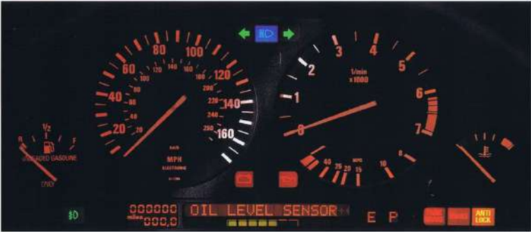
All instruments are directly in the driver's line of sight with large analog dials for primary information such as road speed and engine speed, and digital displays for mileage and secondary information such as the Check/Control system.
