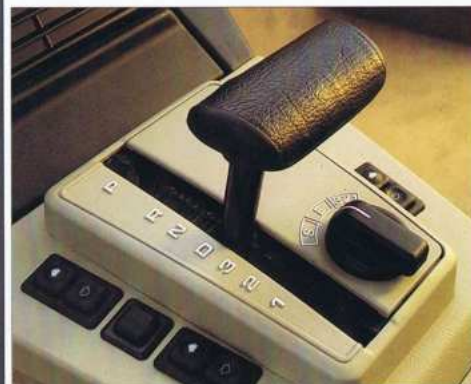
Four-speed automatic transmission (optional) with a special feature: The converter lock-up clutch provides a
