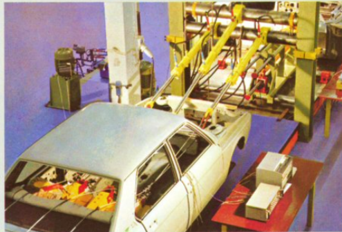
Strength tests of the front panel, seat belt and seat belt anchor points.
