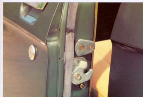
BMW door lock with spherical tumbler and safety wedges – helps eliminate accidental opening during collisions.
