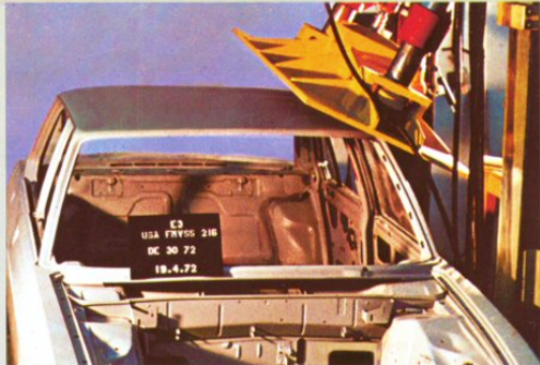
In a simulated turnover, roof strut and roll-bar strength are tested.
