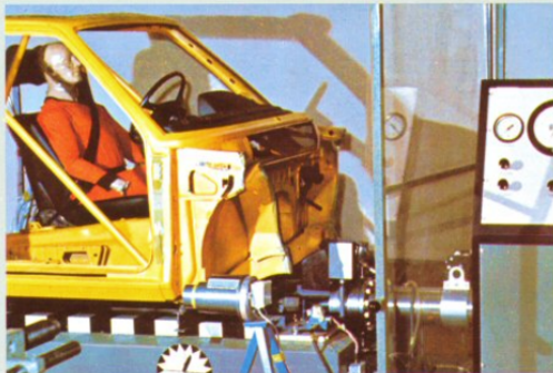
"Sled" used to test cockpit safety equipment.
