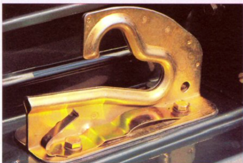
Special hood lock with "catch hook".
