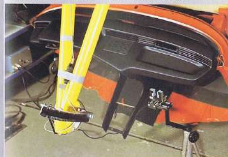
Pendulum impact test of energy absorbing instrument panel.
