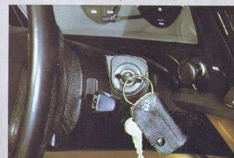
Starter/ignition lock integrated into steering column away from driver's knee, while still unobstructed.
