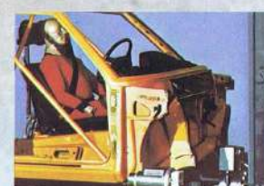
Seat belt system tested on sledge impacts.
