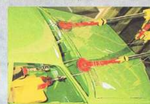
Seat belt anchor-point strength test.
