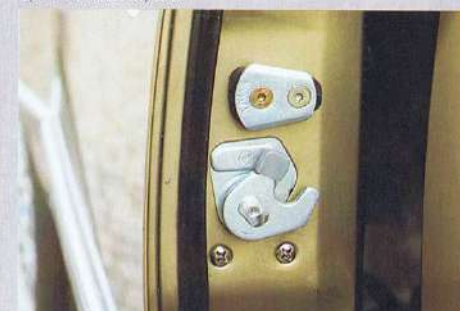
Safety door lock prevents involuntary opening in collision.
