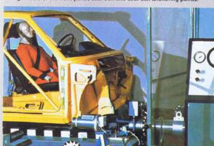
"Sled" used to test cockpit safety equipment.
