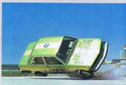
Testing the stability of the passenger safety cell during a lateral roll-over.
