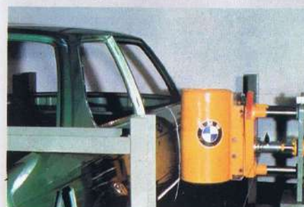
Testing the strength of a side door.
