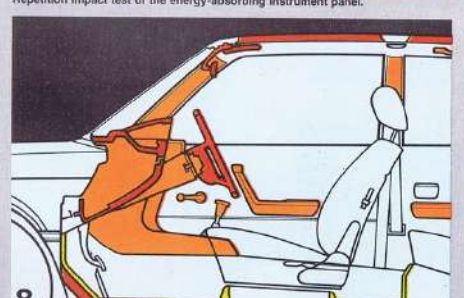
Instrument panel and controls are elastic and deformable.
