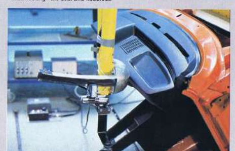
Repetition impact test of the energy-absorbing instrument panel.
