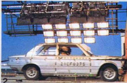
Crash tests to optimize the deformation of the front/rear "crush zones."
