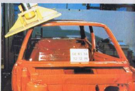
In a simulated overturn, roof strut and roll-bar strength are tested.
