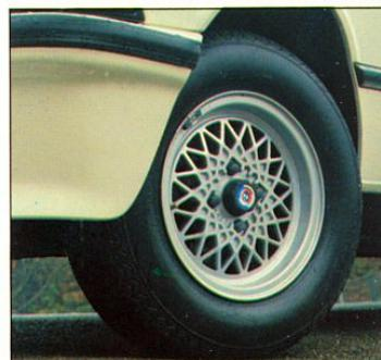
**Above.** **Light alloy wheels.** The light alloy road-wheel has been designed for strength and appearance and has anodised finish for easy cleaning. The Motorsport roadwheel, developed by our motor racing team, is stringently x-rayed before factory release.
