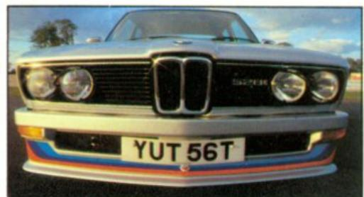
Left. Tough **fibreglass spoilers** have been developed in a wind tunnel for greatly improved performance and high speed stability. Front spoiler reduces drag co-efficient, rear spoiler exerts downward thrust at speed. (Front spoiler only illustrated.)
