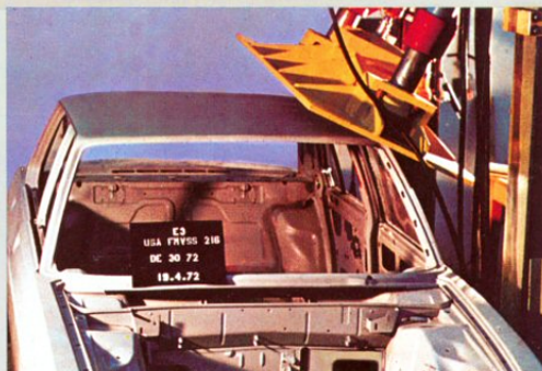
In a simulated turn over roof strut and roll bar strength is tested.
