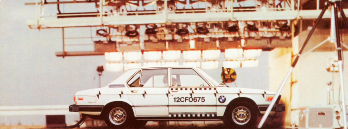
Crash tests to optimize the deformation of the front/rear "crush zones"
