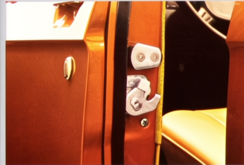
BMW door lock with spherical tumbler and safety wedges – eliminates accidental opening during collisions
