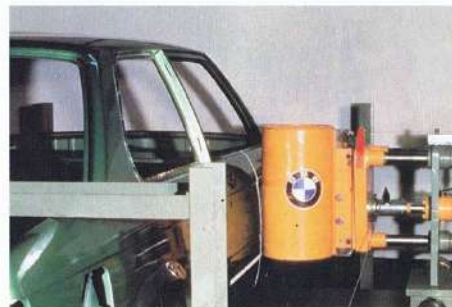
Testing the strength of a side door.
