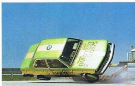
Testing the stability of the passenger safety cell during a lateral roll-over.
