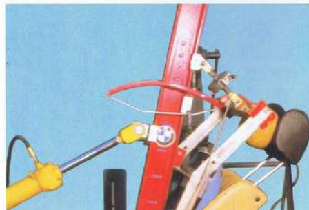
"Load-testing" the seat and headrest.
