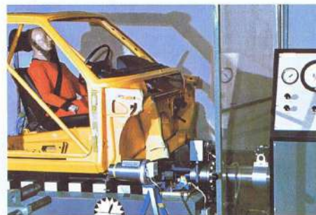
"Sled" used to test cockpit safety equipment.
