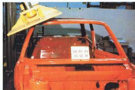
In a simulated overturn, roof strut and roll bar strength is tested.
