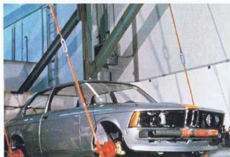
Collision simulation at slow speeds on the "Pendulum".
