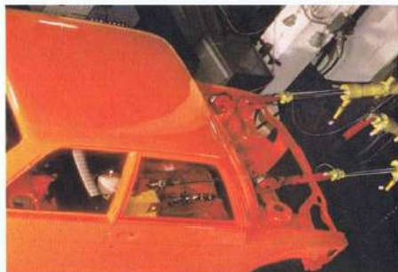
Strength tests of the front panel, seat belt and seat belt anchoring points.
