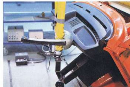
Repetition impact test of the energy-absorbing instrument panel.
