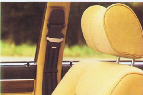
Systematic safety with the standard combination of head restraints and front 3-points inertia reel seat belts.
