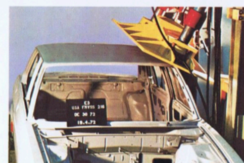
Checking the strength of the roof pillars and roll-over bar if the car overturns.
