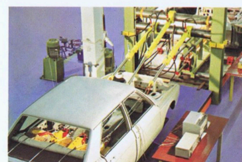
Checking the strength of the bulkhead and the seat and seat belt anchorage points.
