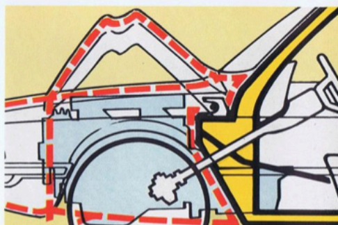
Pre-programmed buckling of bonnet.
