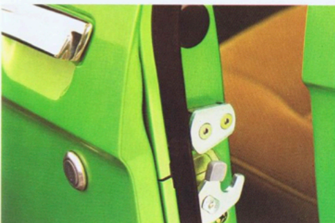
BMW door lock with ball catch and safety anti-burst strikers — do not open on impact.
