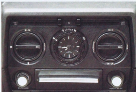
Heating and ventilation system, quartz clock integrated in the rotary switch for the 3-speed blower.
