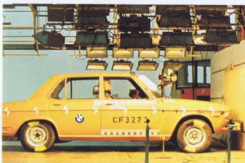
Crash tests to give optimum front and rear collapsing zones.
