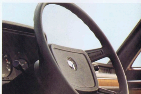
4-spoke safety steering wheel with large padded central boss. (Foam-padded steering wheel as optional extra.)
