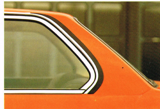
Air extraction through ventilation slots behind the rain guttering on the rear roof pillars.
