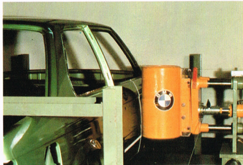
Testing the strength of a side door.
