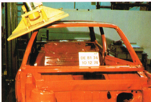
Testing the strength of roof struts and roll-over bars – simulating overturning.
