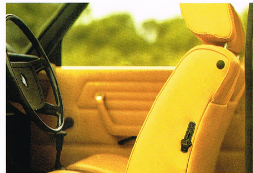
The head-rests are height adjustable in each case. The adjustment is effected by turning the button situated on the left hand side of each seat.
