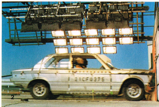
Crash tests to optimise the deformation behaviour of the front and rear vehicle ends.
