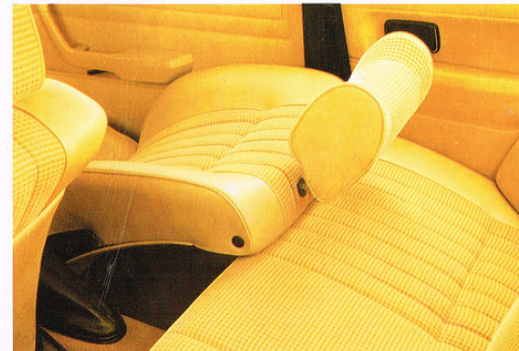
Infinitely adjustable reclining seats, easy seat adjustment on roller bearings.
