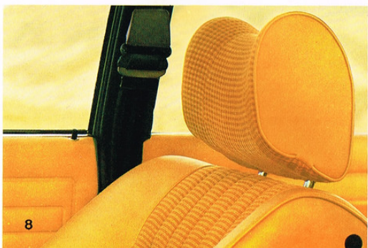
Systematic safety by a standard combination of height-adjustable head rests, adjusted by the touch of a button, and three-point automatic safety belts.
