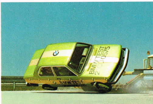
Lateral overturn – testing the stability of the safety cell.
