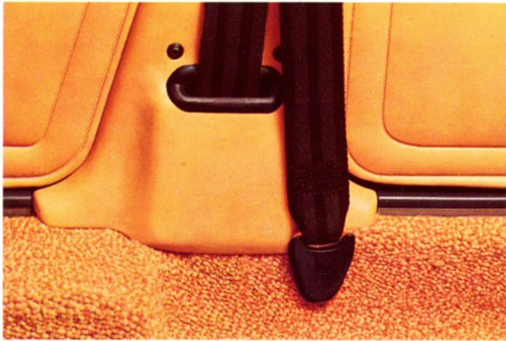
Recessed automatic reel for the 3-point seat belts for front seats.
