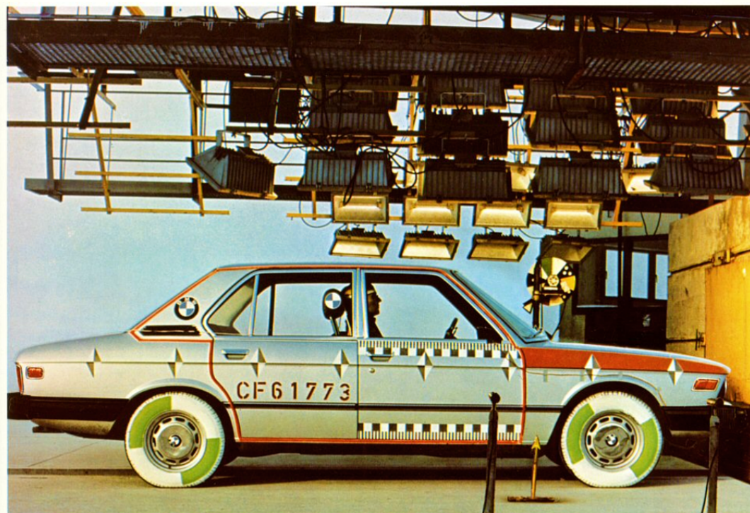
Systematic crash tests for the purpose of optimizing the deformation or crush behavior of front and rear zones.
