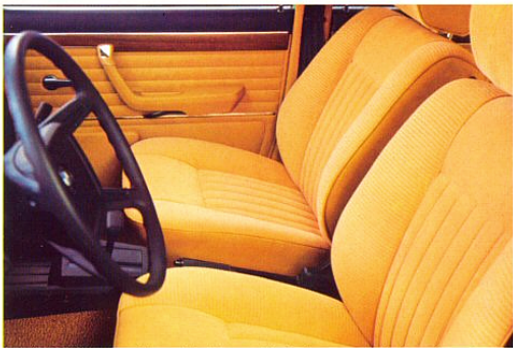
Seats have an orthopedically molded shape, providing firm lateral support, cloth or leatherette upholstery on demand.
