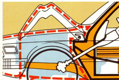
Programmed crush sequence of engine hood with special interception device.
