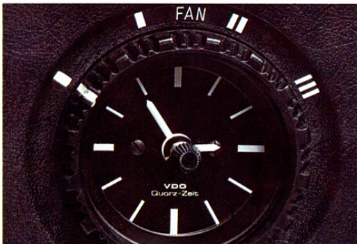
Quartz clock, accurate to plus or minus one second every twenty-four hours.
