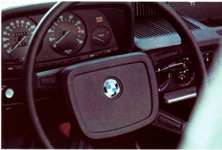
Four-spoke, padded steering wheel with center safety impact pad and four horn contacts.
