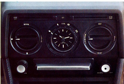
Efficient heating and ventilation system with three-speed blower and individual control ducts.
