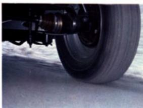
brake operates mechanically on rear wheels
