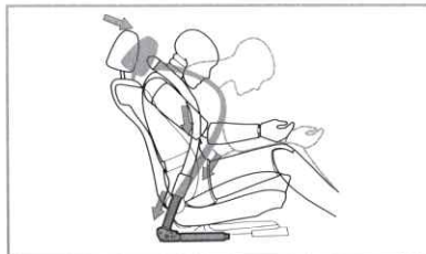
Active Headrests and Safety Belt Pre-Tensioners
