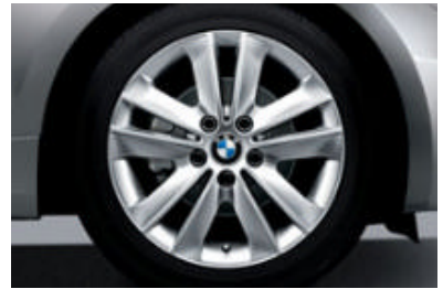
□ SA2KC BMW light-alloy wheels V-spoke 141, 7 J x 17", 205/50 R 17 tyres. (standard for the 120d)
