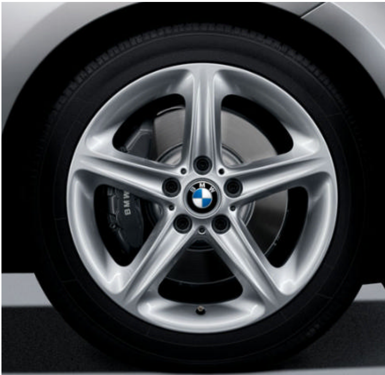
□ SA2SM BMW light-alloy wheels Star-spoke 264 with mixed tyres, 7.5 J x 18" with 215/40 R 18 tyres at the front, 8.5 J x 18" with 245/35 R 18 tyres at the rear (standard for the 135i).
