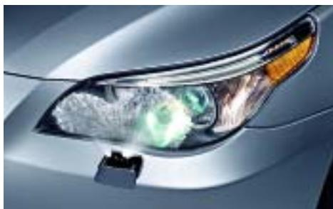
□ **High-pressure liquid headlight cleaning system** helps keep headlights clean of ice, mud, road salt and other coatings, for maximum road illumination and enhanced driving safety. (included in Cold Weather Package)
