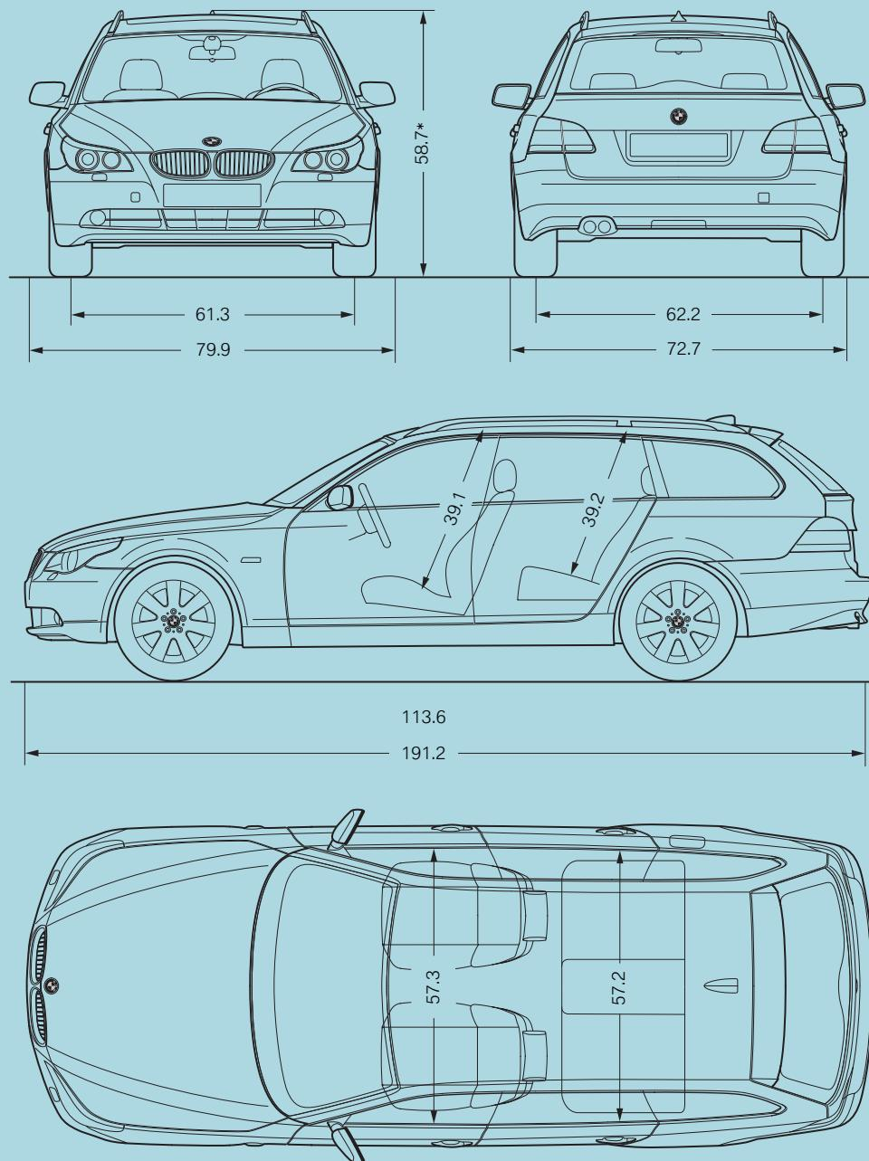
Illustrations above: All dimensions in inches. \*Includes height of roof rails and antenna.
