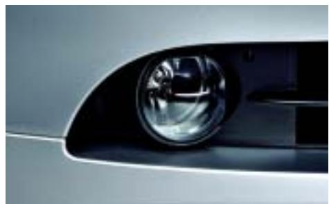
■ **Halogen free-form foglights**, integrated into the deep front spoiler, enhance your margin of safety in bad visibility. Ellipsoid free-form technology provides even light distribution on the road.
