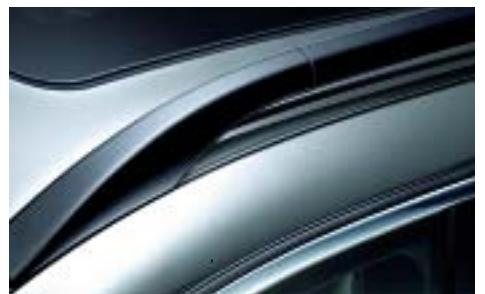
■ **Roof rails** closely hug the lines of the roof. They easily accommodate additional cargo, as well as bicycles, skis, snowboards, etc., when equipped with the multifunctional BMW roof rack system. (Refer to the Original BMW Accessories catalog or visit your authorized BMW center for a full selection.)
