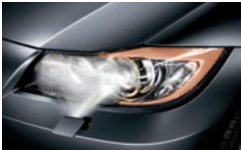
□ **Xenon Adaptive Headlights** provide brilliant clarity of the road ahead and to the side at night and in conditions with poor visibility. The dynamic auto-leveling feature adjusts for varying passenger and cargo loads, helping to keep headlight glare out of the eyes of oncoming drivers. **BMW Adaptive Headlights** provide optimum road illumination around corners and bends by focusing the headlight beam toward where the vehicle is being driven.
