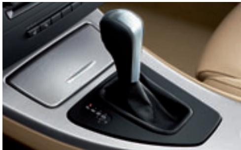
□ **Six-speed STEPTRONIC automatic transmission** provides a choice of three modes: "Drive," which incorporates BMW's Adaptive Transmission Control; "Sport" automatic, for a more dynamic shift pattern; and STEPTRONIC automatic, for the hands-on control of a manual without using a clutch.
