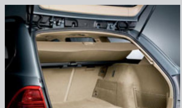
The removable cargo-area cover tilts up automatically when you open the rear window or tailgate.
