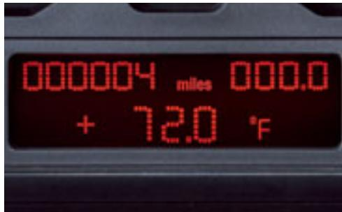
An **on-board computer** offers valuable travel information, with readouts on expected travel range on remaining fuel, average mpg and average speed. An external thermometer sounds a warning when the temperature falls below 38°F – indicating that the road may ice up.
