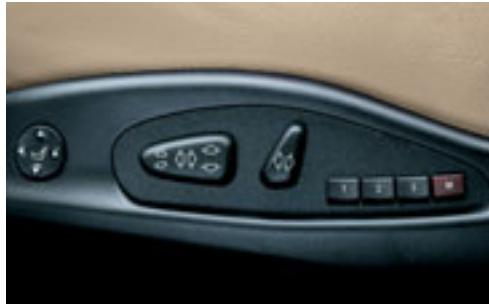
**Eight-way Power front seats** include a **driver's seat and mirror memory system**, which lets up to three drivers set their preferred seat and exterior mirror positions. (Plus, the passenger's-side mirror tilts down when vehicle is shifted into reverse gear.) (330Ci; optional and included in 325Ci Premium Package.) Lumbar support [shown] is included in 330Ci and 325Ci Premium Package)
