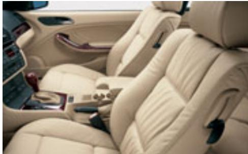
**Eight-way adjustable seats** (including 2-way headrests) firmly support the driver and front passenger over long distances. Front seat bolsters help eliminate “submarining” during sudden stops. (325Ci; 330Ci has eight-way power seats)
