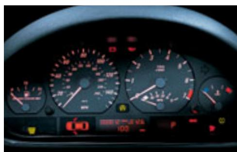
The **instrument panel** presents all important information at a glance through analog gauges and LCD readouts. When parking lights or headlights are on, the gauges are lit in an easy-to-read red.
