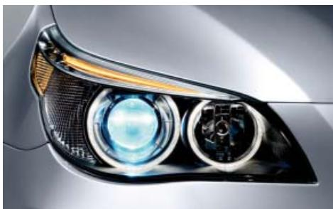
■ **Xenon headlights** illuminate the road ahead and to the side with brilliant clarity. These headlights also feature auto-levelling to adjust for varying passenger and cargo loads. In conjunction with Adaptive Headlights, this also means much improved visibility in bends, as the adjustable headlights are directed into the bend as soon as the vehicle begins cornering.
