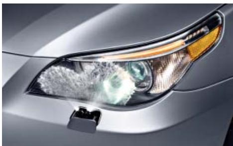
■ **Headlight cleaning system** ensures optimum headlight brightness in all kinds of weather. When the lights are on, the headlights are automatically cleaned in parallel with the windscreens.
