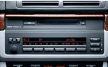
□ BMW Business , 4 x 20 W amplifier output, diversity aerial system (three aerials in the rear window for optimum FM reception), Dolby B/C, scan function, integrated cassette player, connection for BMW CD changer (standard on the 530i, 535i, 540i and 530d).
