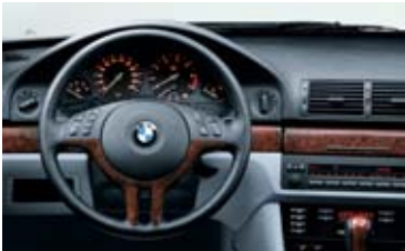
□ Sports steering wheel , 375 mm dia, shown here with optional multifunction control, three-spoke, steering wheel bracket in the same colour as the standard interior trim or in high-quality wood, gearshift lever knob / selector lever handle in leather or wood.
