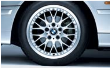
□ BMW light-alloy wheels , cross-spoke styling 42, 8 J x 18" at the front on 235/40 R 18 tyres, 9 J x 18" at the rear on 265/35 R 18 tyres.
