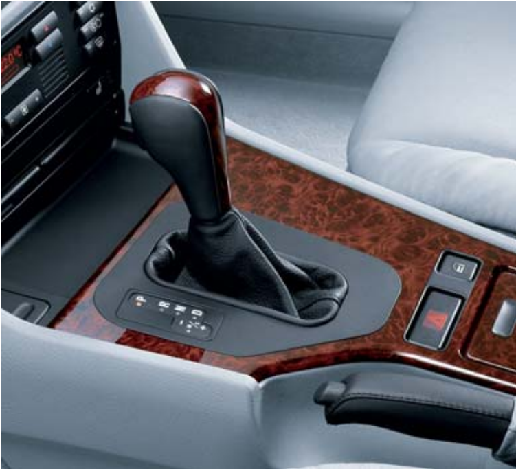
□ Five-speed EH automatic transmission with Steptronic, Adaptive Transmission Management (ATM), Shiftlock/Interlock; Steptronic enables the driver to use the automatic transmission like a manual gearbox without operating the clutch (not on the 520d).
