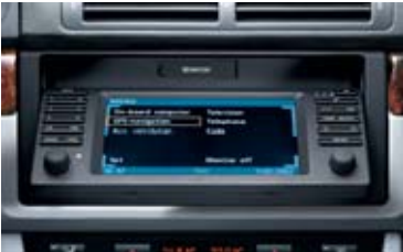
□ Navigation system Professional* with 16:9 on-board monitor (optional TV function) incl BMW Professional radio with cassette player guiding you quickly and accurately to your destination. The split-screen function presents two features on the screen simultaneously, for example your route guidance and another function (data from the on-board computer, radio, etc).
