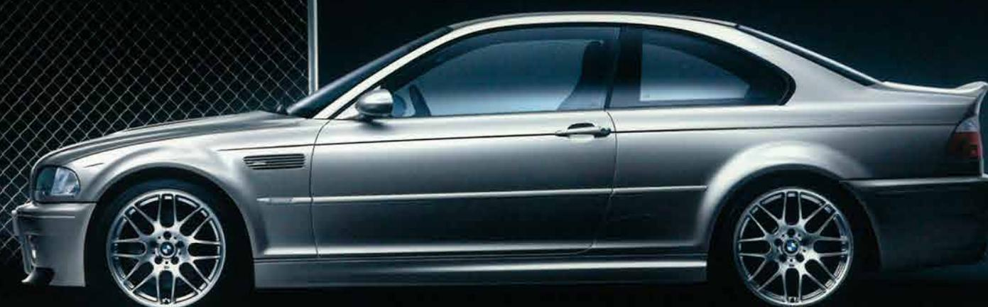
Many sports cars pay homage to Formula 1. The M3 CSL has Formula 1 built in: it's a technological sum of our collected motorsport experience. At this level it's not enough just to save weight by leaving things out. Innovative lightweight technologies must be used to optimise existing components. The roof as well as the front and rear apron are made entirely from carbon-fibre reinforced plastic (CFP), as is the door trim and the centre console. The boot is made of glass-fibre rein-
