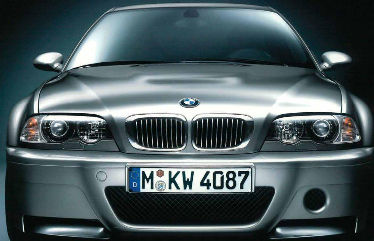
The identifying marks of the M3 CSL: the lightweight aluminium bonnet with powerdome, CFP roof, lightweight synthetic boot lid, aerodynamic flaps on the front CFP bumpers and extra air intake optimised for aerodynamics. Remember them in case you're in the car park rather than the pit.
