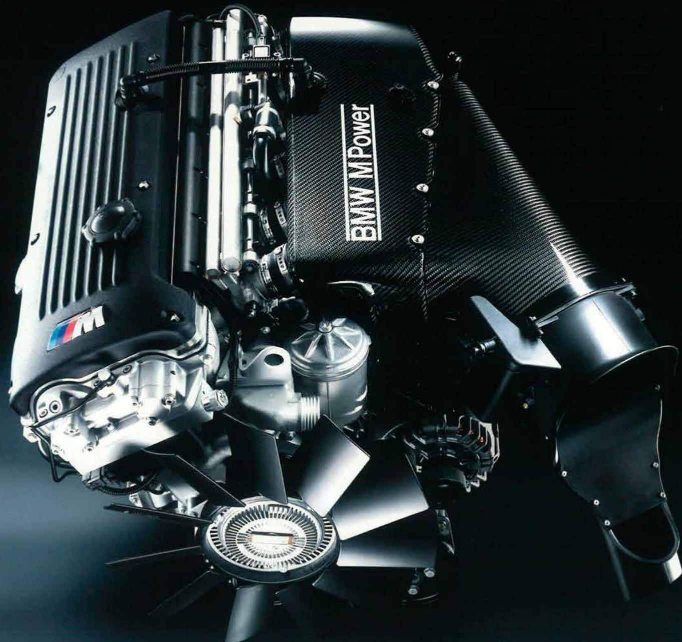
You'll probably want to open the bonnet more than the boot. The facts: 3.25 litre 6-cylinder in-line, 265 kW (360 bhp) at 7900 rpm, maximum torque of 370 Nm at 4900 rpm.
