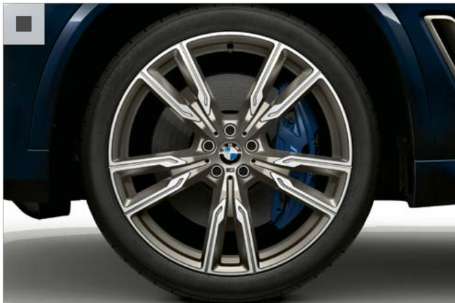
22" M light alloy V-spoke style 747 M wheels, front 9.5J x 22 with 275/35 R22, rear 10.5J x 22 with 315/30 R22 mixed tyres. Standard on the M50i and M50d models.
