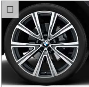
22" BMW Individual light alloy V-spoke style 746 wheels, front 9.5J x 22 with 275/35 R22, rear 10.5J x 22 with 315/30 R22 mixed tyres. Also available with the M Sport Plus Package on M Sport models.
