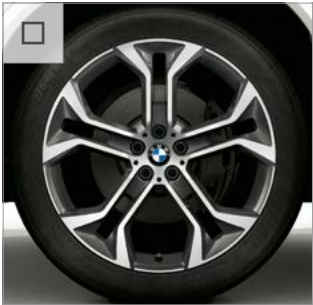
21" light alloy Y-spoke style 744 wheels, front 9.5J x 21 with 275/40 R21, rear 10.5J x 21 with 315/35 R21 mixed, run-flat tyres. Optional on xDrive40i and xDrive30d Sport models.
