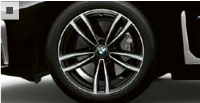
19" M light alloy Double-spoke style 647 M wheels in Bicolour, with run-flat tyres, front 8.5J x 19 with 245/45 R19 tyres, rear 9.5J x 19 with 275/40 R19 tyres. Standard for M Sport models.
