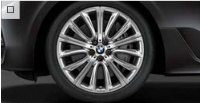
20" light alloy V-spoke style 628 wheels, Bicolour with run-flat tyres, front 8.5J x 20 with 245/40 R20 tyres, rear 10J x 20 with 275/35 R20 tyres. Optional for SE models.
