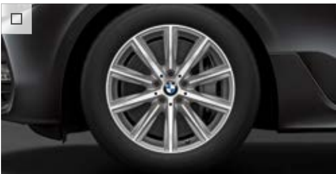
18" light alloy V-spoke style 684 wheels with run-flat tyres, 8J x 18 with 245/50 R18 tyres. Optional for SE models.
