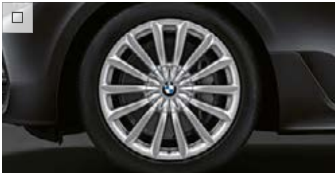
19" light alloy V-spoke style 620 wheels with run-flat tyres, front 8.5J x 19 with 245/45 R19 tyres, rear 9.5J x 19 with 275/40 R19 tyres. Optional for SE models.
