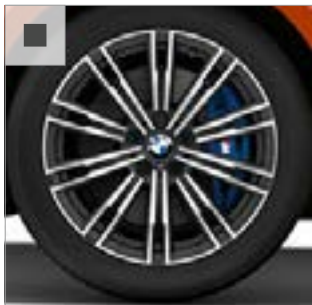
18" M light alloy Double-spoke style 790 M wheels, Bicolour Orbit Grey, front 7.5 J x 18 with 225/45 R18, rear 8.5 J x 18 with 255/40 R18 run-flat tyres. Standard on M Sport models. Optional on M340i/d xDrive models. Non-run flat tyres standard for 330e M Sport model.
