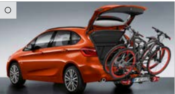
The foldable Compact rear bike rack is light but sturdy and can carry up to 60kg. It can be quickly and securely mounted on the tow ball and transport up to two bicycles or e-bikes. When folded up, it can be stored in the luggage compartment tray, safe from spray and protected in the event of a collision.
