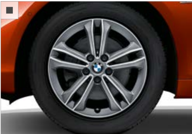
17" light alloy Double-spoke style 549 wheels, Orbit Grey, 7.5J x 17 with 205/55 R17 tyres. Standard for Sport models.
