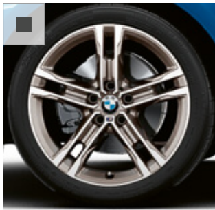
18" M light alloy Double-spoke style 556 M wheels, Bicolour, Cerium Grey matt, 8 J x 18 with 225/40 R18 tyres. Standard on the M135i xDrive model.
