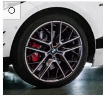
Weight-optimised 19" M Performance light alloy Double-spoke style 555 M wheels in Bicolor Jet Black. TPMS summer complete wheel set.
