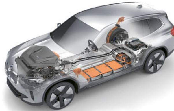
► Electric motor of the newest generation: The drive in the new BMW iX3 manages completely without rare earth metals.
