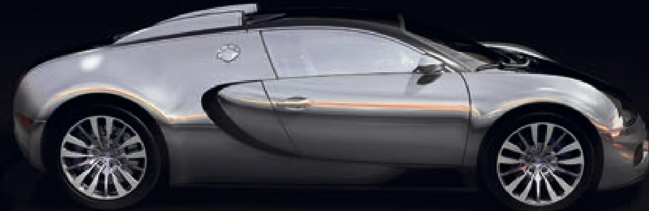
The EB 16.4 Veyron Pur Sang is a two-tone study of pure material showing the car's true essentials: carbon and aluminium. The clear-coated carbon monocoque holds the engine and the passenger cell, while the polished aluminium panelling is enhanced by reflections in the sculpted bodywork.
