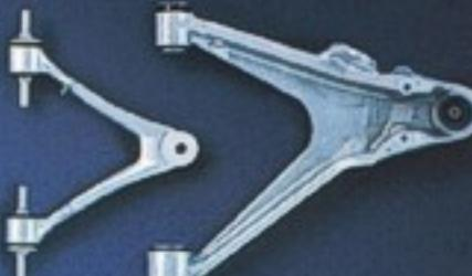
New bushing technology and applications have enhanced the balance between ride and handling.
