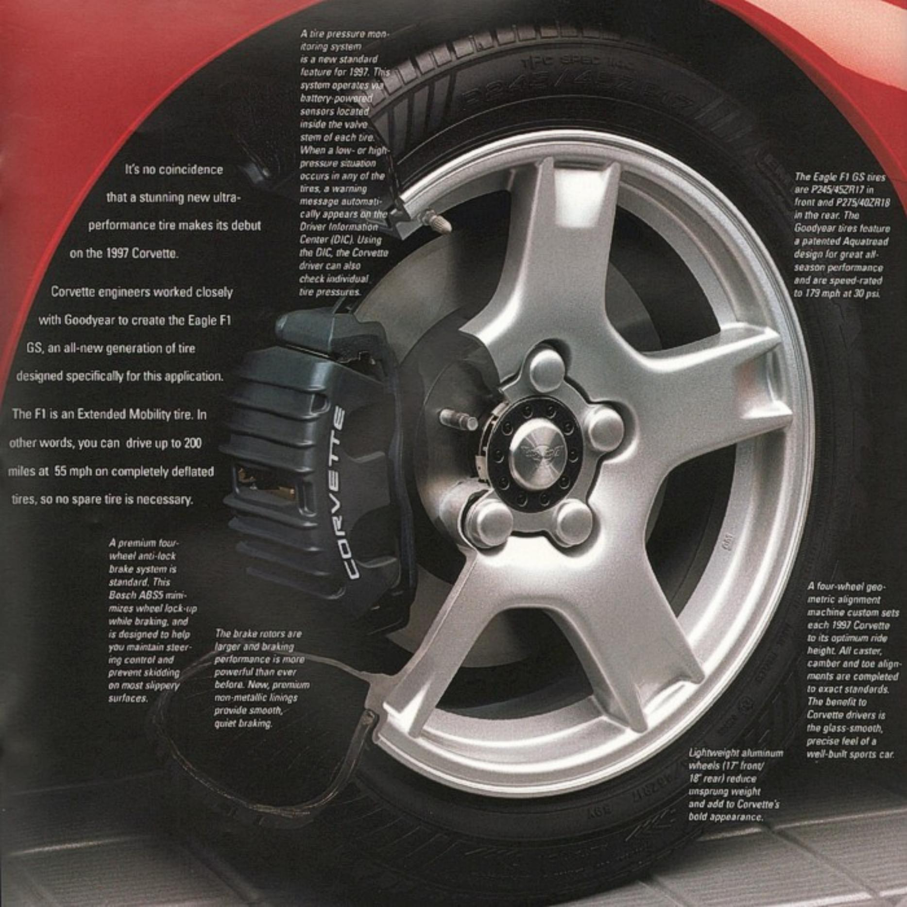
A tire pressure monitoring system is a new standard feature for 1997. This system operates via battery-powered sensors located inside the valve stem of each tire. When a low- or high-pressure situation occurs in any of the tires, a warning message automatically appears on the Driver Information Center (DIC). Using the DIC, the Corvette driver can also check individual tire pressures.
