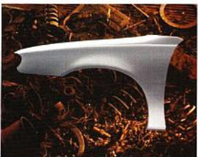
For durability and long life, all of Malibu's exterior body panels are precision-stamped from corrosion-resistant 2-sided galvanized steel.
