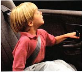
For your peace of mind, Malibu's rear door locks can be set to prevent the doors from being opened from the inside.
