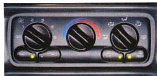
Rotary controls for the standard air conditioning system have been designed for easy, almost intuitive use. To protect the ozone layer, Malibu's air conditioning uses a non-CFC refrigerant.
