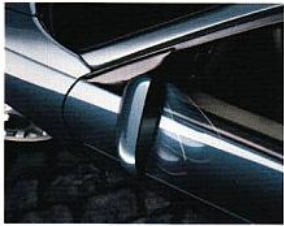
Malibu's dual outside rearview mirrors are designed to "break away" on impact to help protect pedestrians, then snap back into position undamaged.
