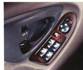
Power windows include a driver's express-down feature for convenience and a passenger window lock-out for safety. Standard on Malibu LS.
