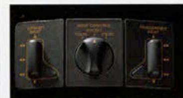
Standard Selective Ride Control allows the driver to select one of three system settings (Touring, Sport or Perf) by rotating a switch on the console panel (above). Each setting provides six different shock absorber damping levels — depending on vehicle speed (see chart at left).
