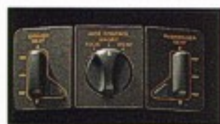
Standard Selective Ride Control allows the driver to select one of three system settings (Touring, Sport or Perf) by rotating a switch on the console panel (above). Each setting provides six different shock absorber damping levels — depending on vehicle speed (see chart at left).
