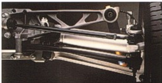
A sophisticated five-link independent rear suspension is standard on Corvette.
