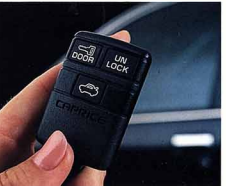
Optional Keyless Entry allows you to lock or unlock your doors, and unlock trunk from up to 30 feet away.
