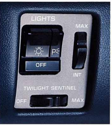
Optional Twilight Sentinel. Automatically turns lights on and off. Includes delay timer feature that allows you to keep headlights lit for up to 3 minutes after you leave car.
