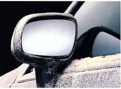
Optional dual heated electronic remote mirrors stay clear at the touch of the rear defogger switch.
