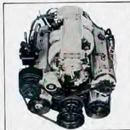
5.7 Liter V8 with Tuned-Port Injection (optional on Camaro IROC-Z Coupe).
