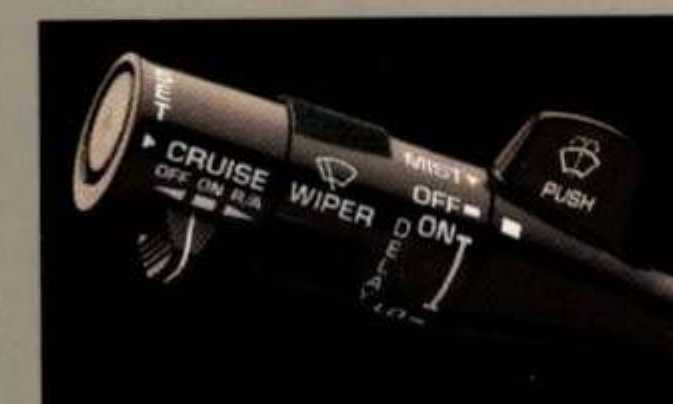
Convenient electronic speed control has accelerate/decelerate and resume features.
