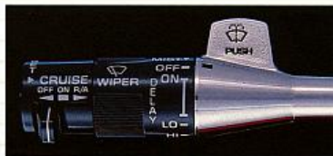
Electronic speed control and intermittent wiper shown on standard multi-function switch.
